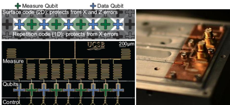
Figure 4. Superconducting quantum computing approaches. (left) Circuit-model computing approach with 9 qubits for error correction ([Martini's group, Google](#)). (right) 3D cavities have enable record coherence times and error correction ([Yale](#)).
