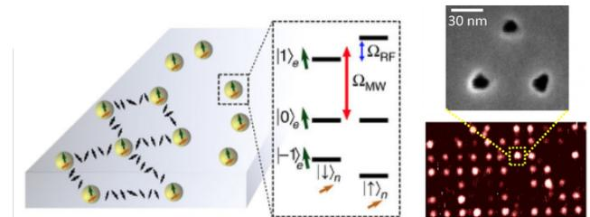
**Figure 11. Arrays of NV-centers in diamond, closely enough spaced so that electron spins interact magnetically, are promising for mid-scale quantum computers that could even function at room temperature. The image on the left shows a schematic of the required architecture (Image credit: N. Yao, *NComm*, 2012); it is now becoming possible to reach the required length scales experimentally (D. Scarabelli, *Nano Letters*, 2016).**
