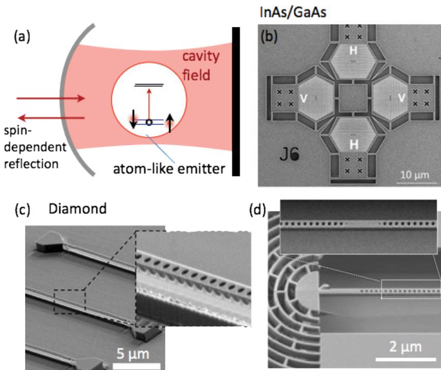
**Figure 10. Optical cavities can act as efficient interfaces between incident photons and atom-like quantum memories (a). Such interfaces based on photonic crystal cavities are being used to link quantum memories in photonic circuits. (b) Cavity-waveguide networks for InAs/GaAs quantum dots. (Credit: Waks group, University of Maryland). (c) Diamond cavity-waveguide systems with triangular (bottom left) and (d) rectangular (bottom right) nanobeams for NV and SiV memories. (MIT and Harvard)**
