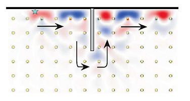
Figure 9. Topologically protected one-way waveguide in which electromagnetic radiation can maneuver around obstacles because backscattering is completely suppressed (*Wang et al. PRL 100 13905 (2008)*).
