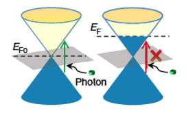
Figure 11. Intercalation of lithium ions in graphite changes the *fermi level* of the electrons and dramatically changes the optical transmission of the film (*Bao et al. Nature Comms. (2014)*).
