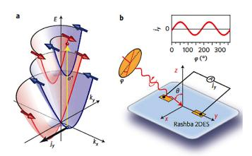
Figure 10. A non-uniform distribution of photoexcited carriers in k-space by circularly polarized light results in spin polarized photocurrent (Yuan et al. Nature Nano., 851-857 (2014)).
