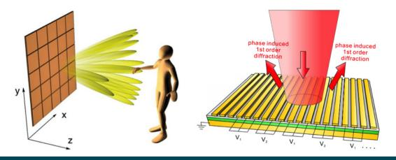
Figure 6. (Left) Metasurface based holographic imaging (Hunt et al., J. Opt. Soc. Am. A 31, 2109 (2014)). A pseudorandom multi-frequency beam pattern formed by a metasurface allows for 3D spatial imaging of the target. (Right) Electric-field-effect tunable conformal optical phased array metasurface (Huang et al., arXiv 1511.09380 (2015))—beam steering is due to electrically induced phase delay between the array elements.
