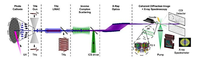
Figure 3. Design for a tabletop X-ray source with nanostructured photocathodes as a source of electrons. The system has intrinsic attosecond synchronization and requires only picosecond lasers at the 1J-level for kHz operation (*Nanni et al. Nature Comms. (2015)*).
