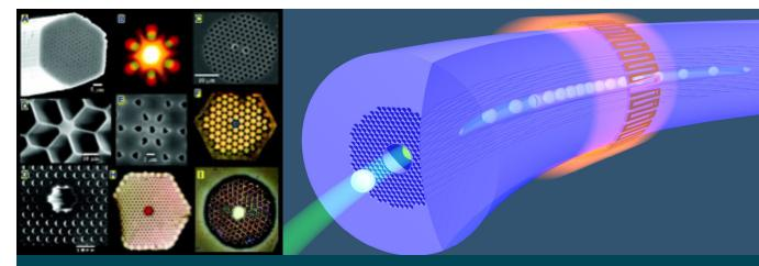
Figure 5. Photonic crystal hollow-core fibers that confine very large power densities, enhance nonlinear interactions, and improve phase matching (*Russell, Philip Science, 358-362 (2003)*). An ionized gas that acts as the *gain medium* can be contained in the core (*Dholakia et al. Physics 5, 76 (2012)*).
