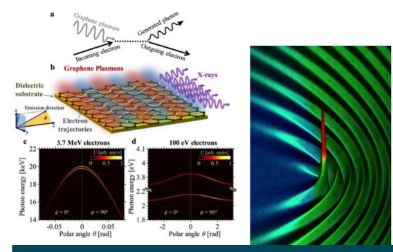
Figure 4. Theoretical design for a graphene plasmon-based free-electron IR to X-ray source. Surface plasmons undulate the electrons and replace the series of magnets in more traditional X-ray sources (*Wong et al. Nature Photonics*, 46-52 (2016)).
