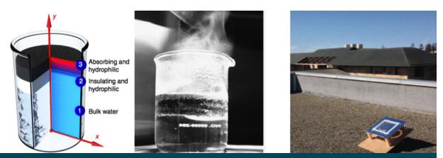
Figure 2. (Left) Solar steam generation by heat localization (Ghasemi et al. Nat. Comms 5, 4449 (2014)). (Right) Passive radiative cooling under direct sunlight (Raman et al. Nature, 515, 7528 (2014)).
